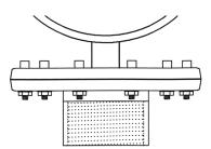
100mm Chamber: Up to 1.5" BSP or NPT 152mm Chamber: Up to 3" BSP or NPT
